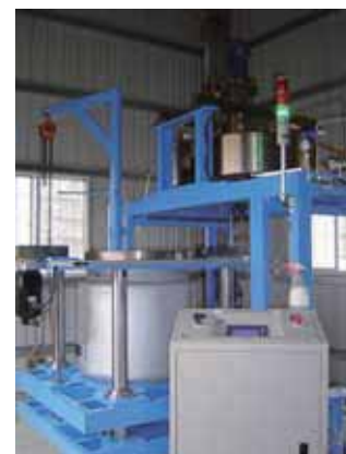
Subcritical Water Biomass Treatment System (24MPa/350°C, 100L)
