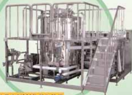
超音波量產型1000L萃取設備 Ultrasonic Mass Production 1000L Extraction Equipment
