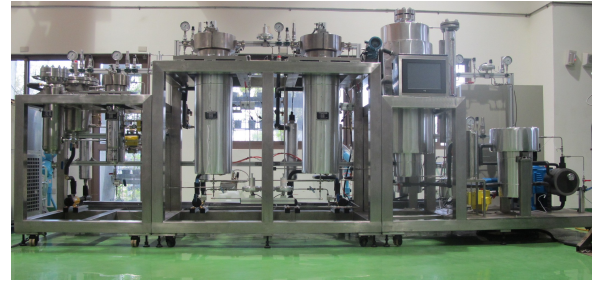
20Lx2x40MPa SCCO 2 Extraction System
