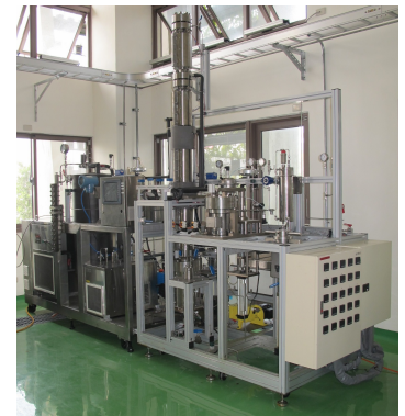
2LPHx35MPa SCCO 2 Fractionation System
