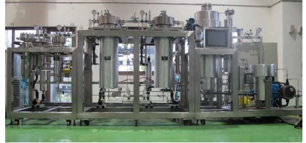
20Lx2x40MPa SCCO 2 Extraction System
