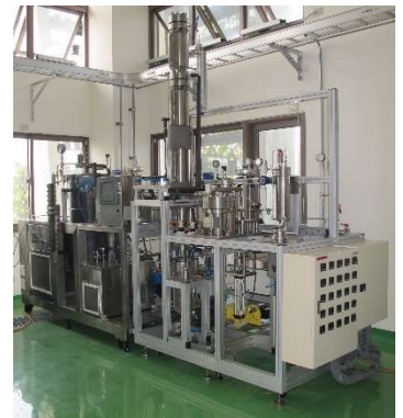
2LPHx35MPa SCCO 2 Fractionation System
