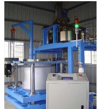
Subcritical Water Biomass Treatment System (24MPa/350°C. 100L)
