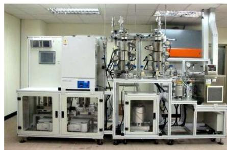
25MPa/480°C Supercritical Fluid Tubular reactor System
