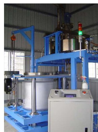
Subcritical Water Biomass Treatment System (24MPa/350°C, 100L)
